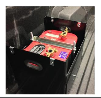
4.1 Place Battery in Box. Fit battery clamp with 2 x M8 L bolts, 2 x M8 Flat Washers and 2 x M8 Nyloc nuts.
