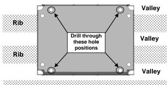
2.3 Mark hole positions of battery box onto vehicle tub.
