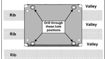
2.15 Mark hole positions of battery box onto vehicle tub.
