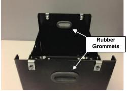
1.2 Install 2 x Rubber Grommets as shown.
