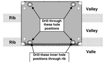
2.27 Mark positions of battery box holes onto vehicle tub.
