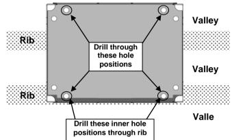
2.39 Mark positions of battery box holes onto vehicle tub.
