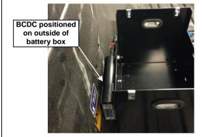
1.3 Install suitable BCDC (if required) using slots as shown
