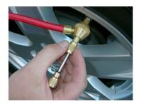
1. With the slide valve pushed forward, thread the valve stem adaptor onto the valve stem in a clockwise direction.
