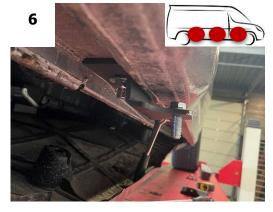
Place screw on bracket first Place bracker on the vehicle and tighten with nut + rivet
